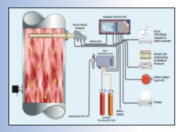
The calculated concentrations can be displayed on a PC or weatherproof industrial PC. Up to four analysers can be connected to the control system with inputs for other instruments such as opacity, velocity and oxygen. The data can be transmitted to the DCS in analogue or modbus formats.
